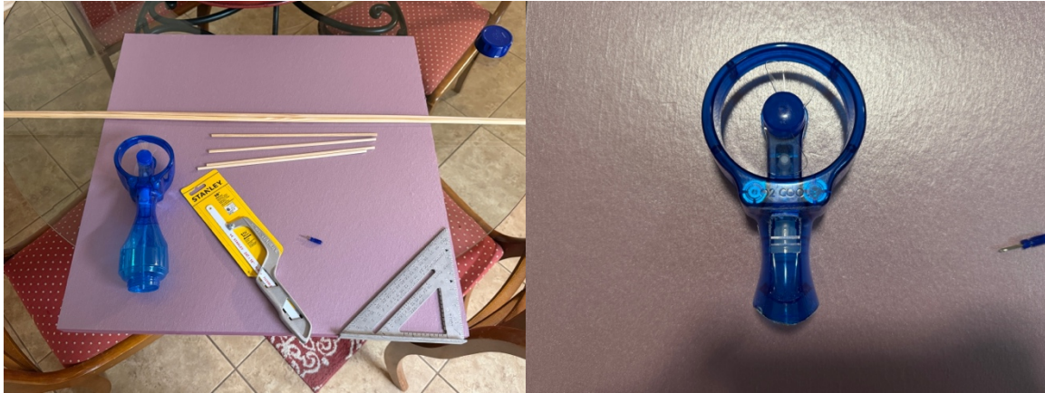
Figure 13. Raw materials for the foam hull proof-of-concept, including insulation foam, handheld fan sprayer, and cutting tools (left), and close-up view of the fan sprayer after modification (right).
