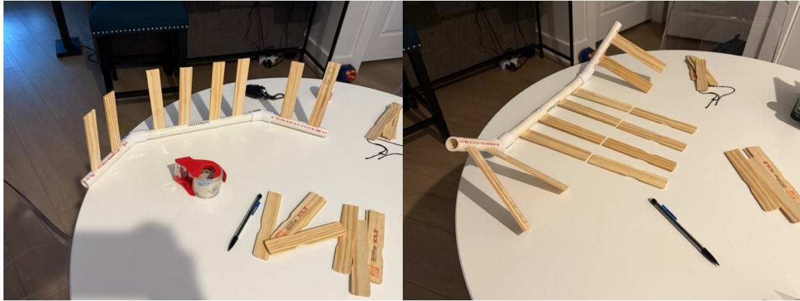
Figure 11. Wooden paint-stick teeth taped in place along the PVC crossbar during initial spacing trials (left) and the secondary angled support members to establish the intended rake geometry (right).
