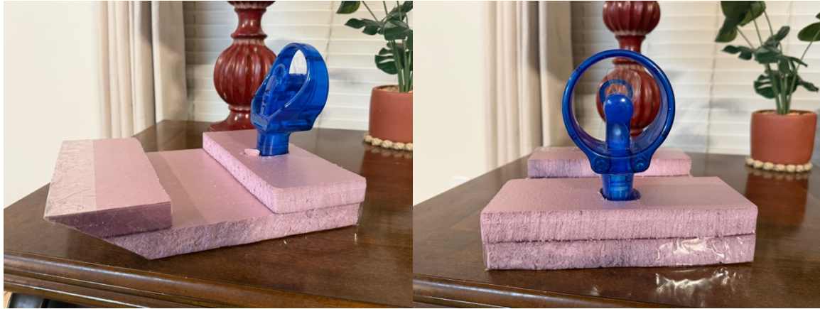
Figure 15. Completed low-fidelity foam hull proof-of-concept featuring the mounted fan sprayer and stepped deck geometry (left) and rear-facing view of the assembled prototype showing fan alignment and hull profile (right).
