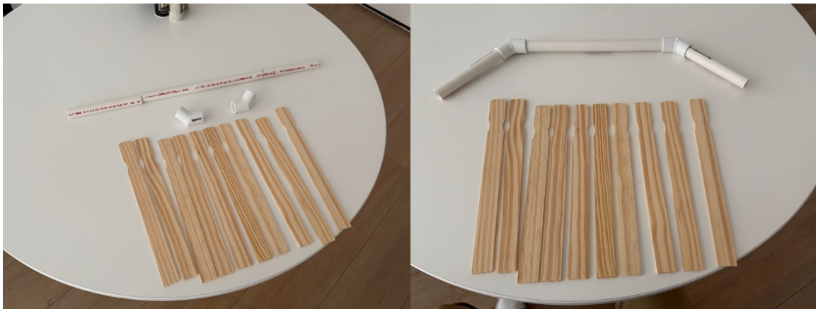
Figure 10. Raw materials for the comb prototype (left) and the assembled PVC support frame (right).
